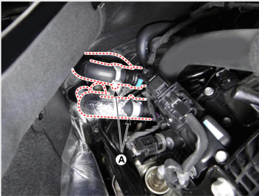
13. Remove the water inlet pipe (A).
