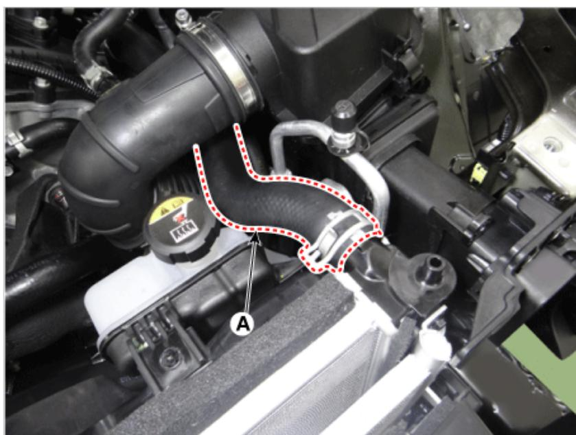
13. Remove the water outlet pipe (A).
